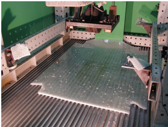
Fig. 10 Broken Standard PVB laminate collapsed at +50°C
