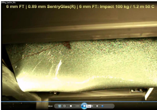
Fig. 3 Ionomer laminate provided "Fall Through" resistance, view from below during the impact
