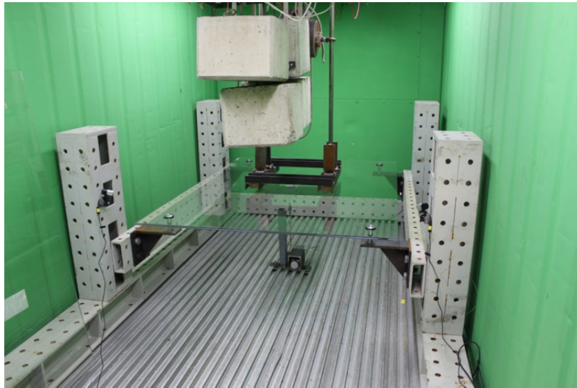
Fig. 7 Post Breakage Test layout in climate chamber
