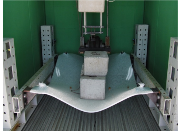
Fig. 13 1.52mm Ionomer laminate collapsed at 300Kg at +50°C
