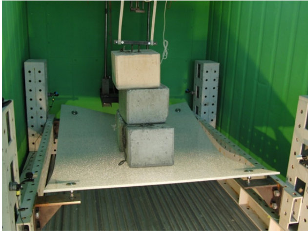
Fig. 8 400Kg load on Ionomer laminate at +21°C
