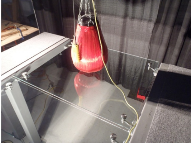
Fig. 2 (a & b) Impact Test on a Frameless (point supported) canopy application, view from above showing the impactor before the impact (a) and a close-up picture of the rotule type fixation system
