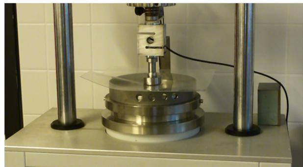
Fig. 13 Imperfection of glass sample and set-up.
