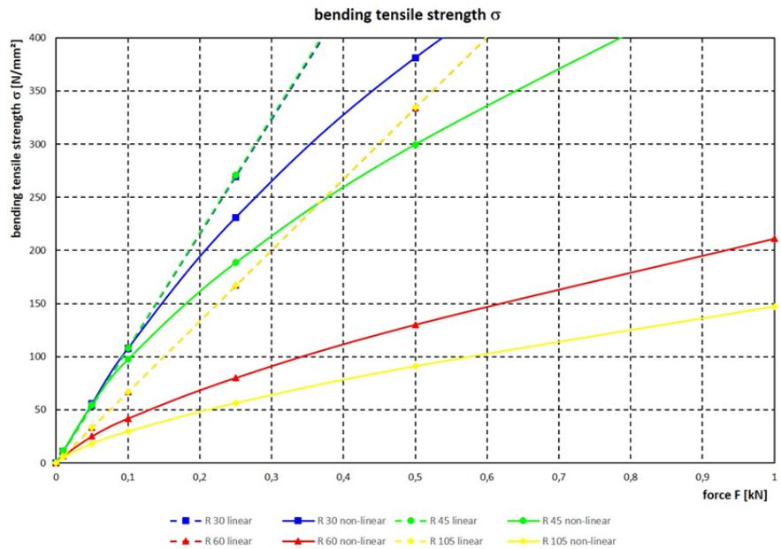
Fig. 11 Diagram - bending tensile strength  $\sigma$  /force F .
