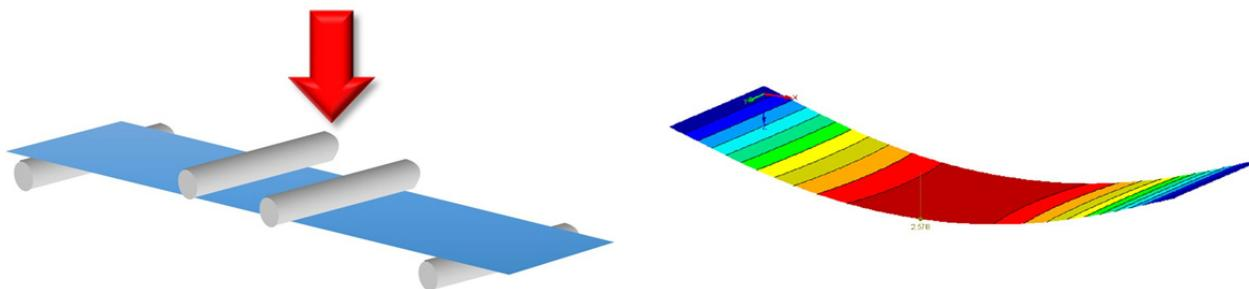
Fig. 6 Four-point bending principle test set-up, deflection of test specimen.
