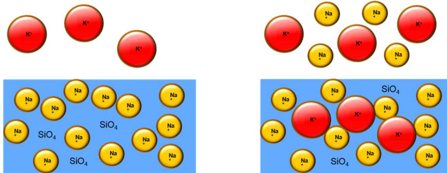
Fig. 3 Chemical treatment – Ionic Exchange.
