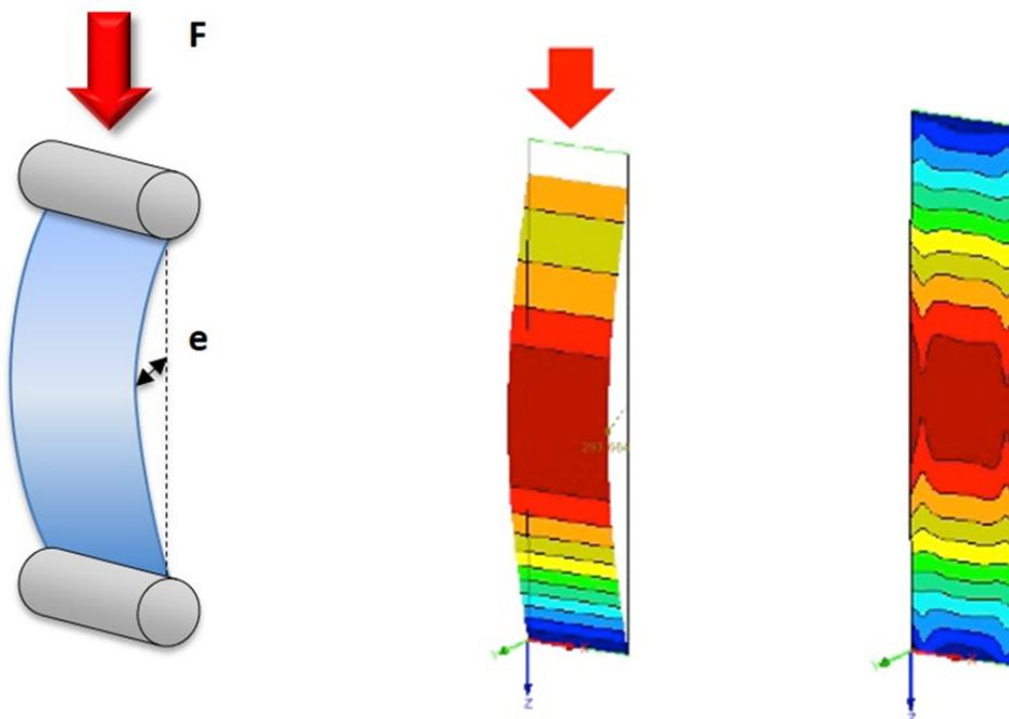
Fig. 8 Principle test set-up for bending in-plane force, deflection and stress distribution.
