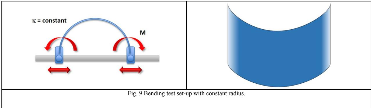
Fig. 9 Bending test set-up with constant radius.
