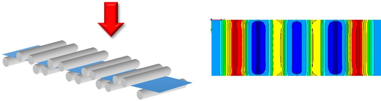
Fig. 7 Multi-point bending test set-up, stress distribution.
