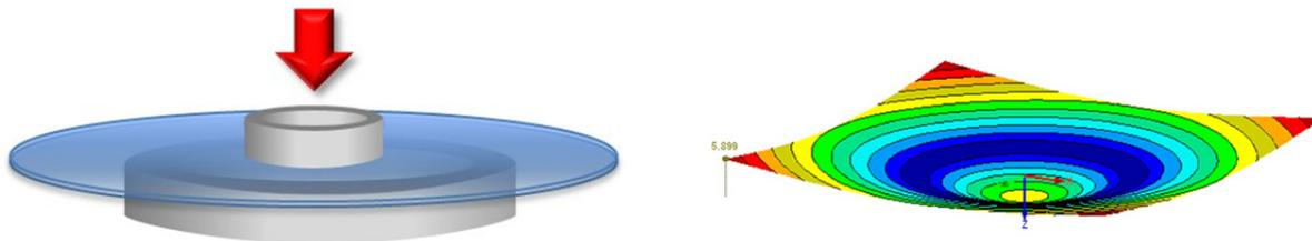
Fig. 4 Ring on ring test set-up, deformation of glass sample.
