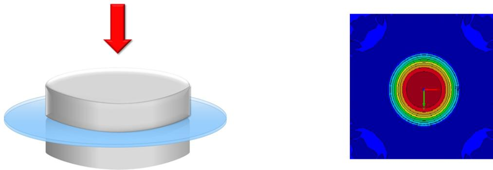
Fig. 5 Pressure pat on ring test set-up, distribution of principle stress.
