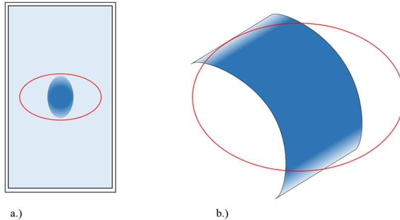
Fig. 12 Area of homogeneous maximum principle stress of simply supported a.) flat glass, b.) cold bent cylindrical glass (semicircle).
