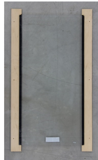
Fig. 3 Prepared specimen with two long joints made from adhesive C – DP490
