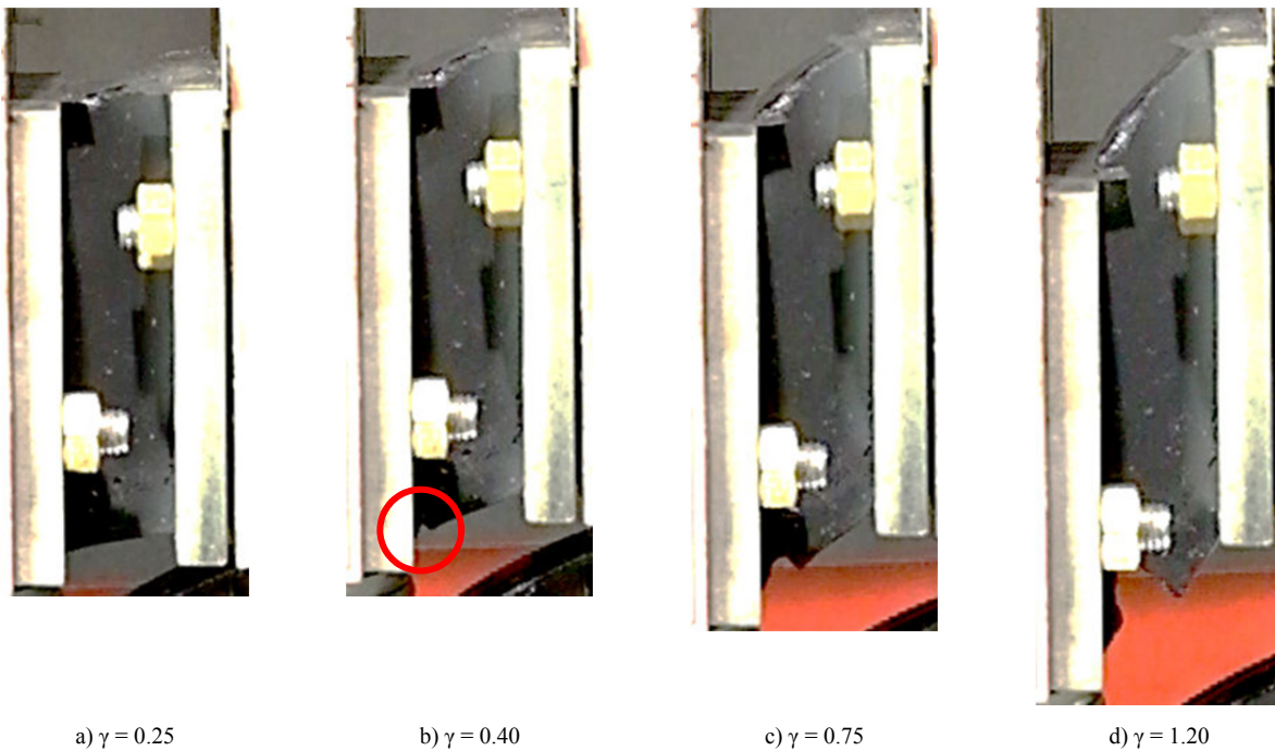
Fig. 16 Observed deformations for the points given in figure 15. \gamma is the engineering shear strain.
