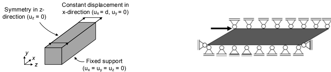
Fig. 19 Applied boundary conditions for the numerical model. Only the silicone sealant is modelled due to the high rigidity of the adherends compared to the sealant.
