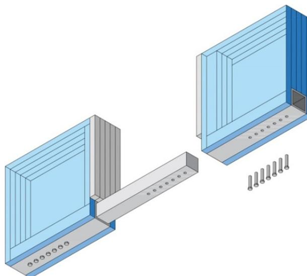
Fig 5 Transfer of tensile force by an internal coupling pin, bolted to the bottom of the reinforcement.
