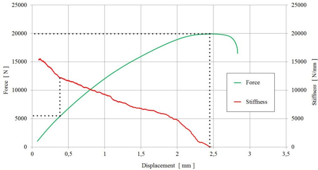
Fig. 6 Force - displacement curve of the Monel alloy 400 specimen, including its derivative.
