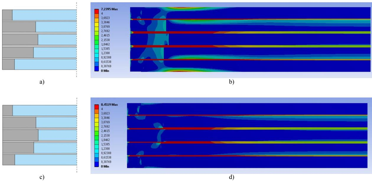
Fig. 3 Maximum principle stress [MPa] caused by thermal contraction after lamination, for two different profiles.
