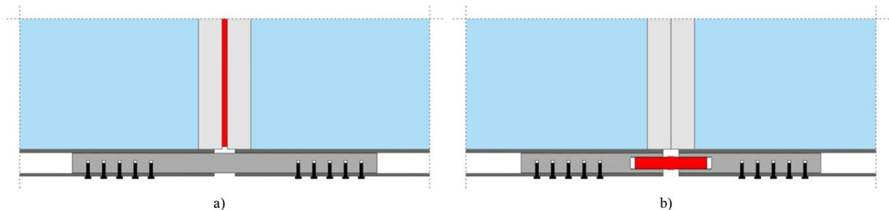
Fig. 9 Solutions to get rid of the clearance between the segments.
