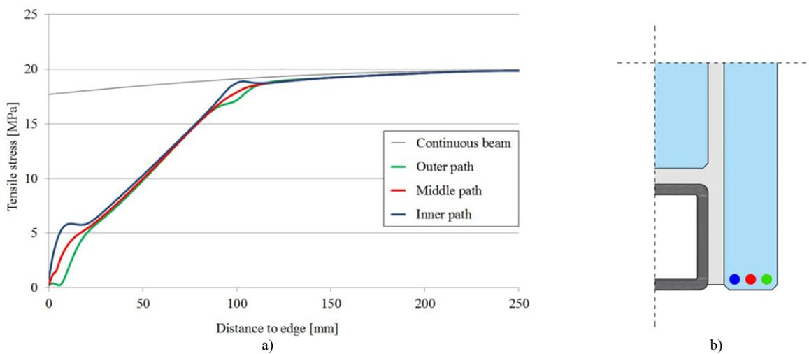
Fig. 10 Tensile stress collected along three different paths.
