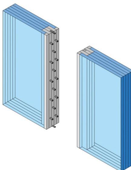
Fig. 2 Transfer of shear force between the profiles, by dowel pins.
