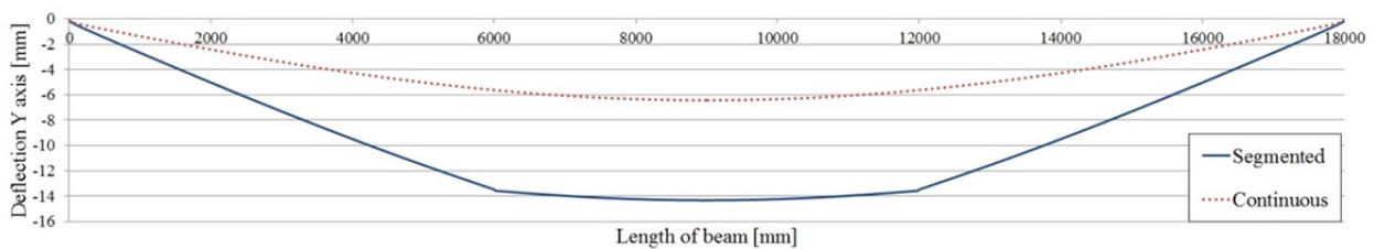
Fig. 8 Vertical displacement of a continuous and the segmented beam.
