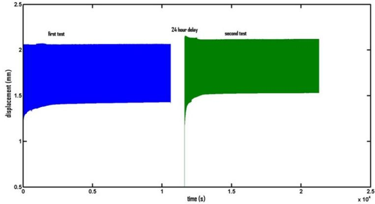
Fig. 5 Results of test with a hold time of 0.1 s and interruption of 24 hours in the middle of the test.
