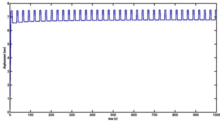
Fig. 6 Initial cycles of test with a hold time of 5 seconds at maximum and 20s at minimum load.
