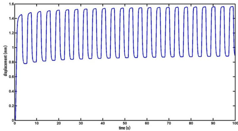
Fig. 8 Initial cycles of test at 40°C with a hold time of 1s.
