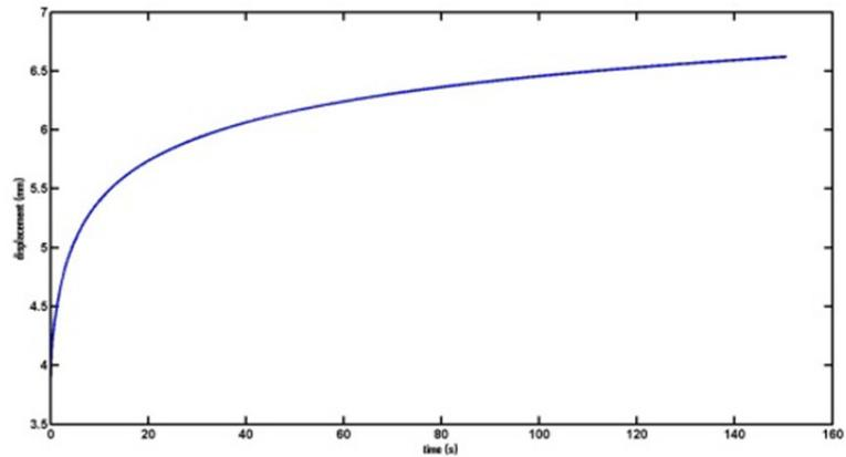
Fig. 4 Creep at 6000N load
