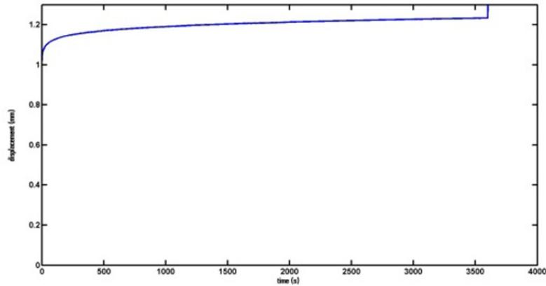
Fig. 3 Creep at 4000 N load
