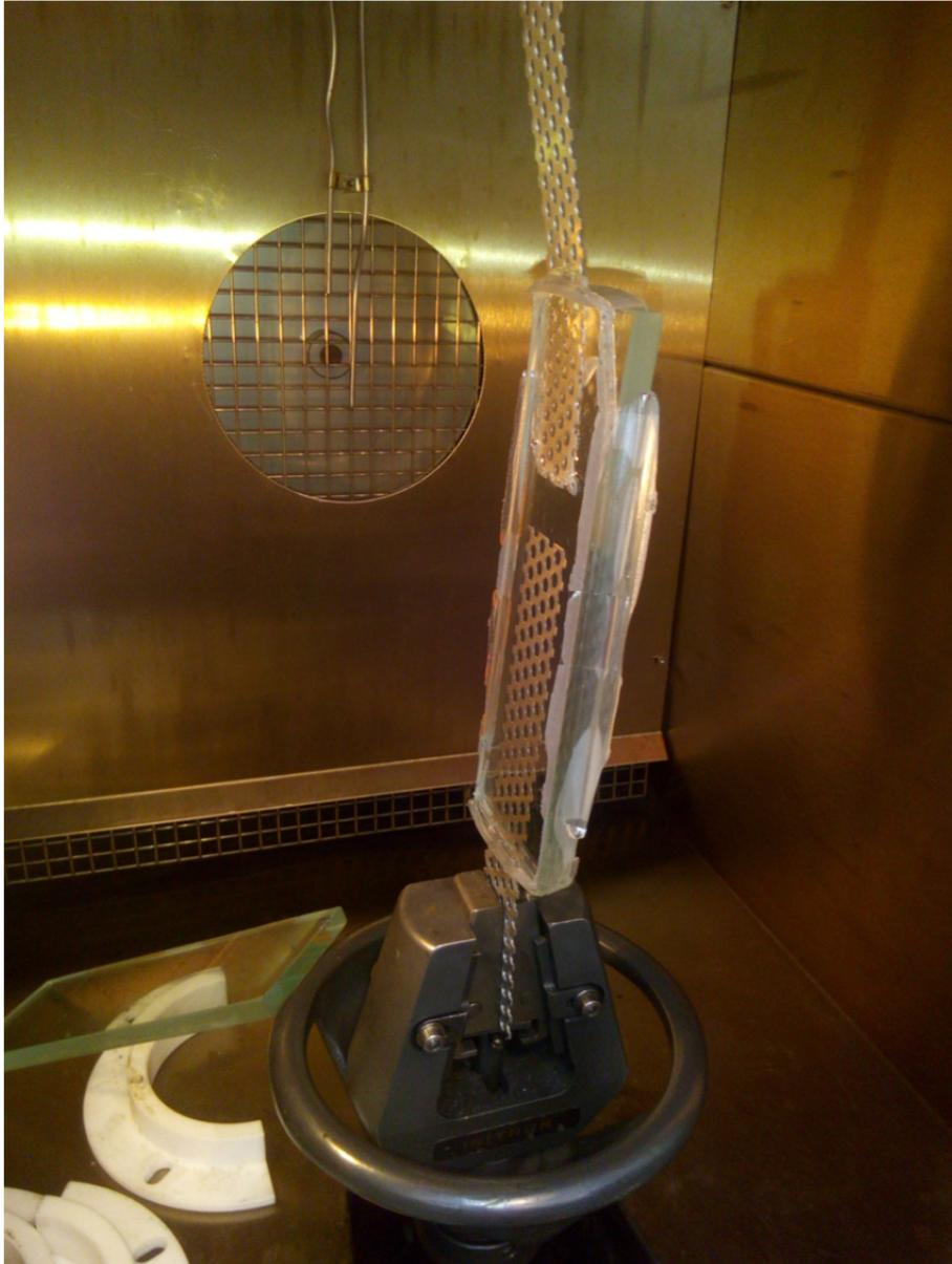
Fig. 13 Specimen 4 after testing at 40°C
