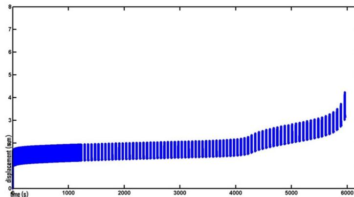
Fig. 11 Results of full test at 40°C with a hold time of 5s at maximum and minimum load.
