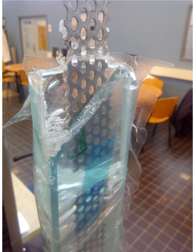
Fig. 2 Specimen after tensile test
