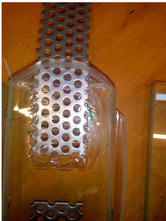
Fig. 14 Pulled out stainless steel of specimen 3 tested at 40°C
