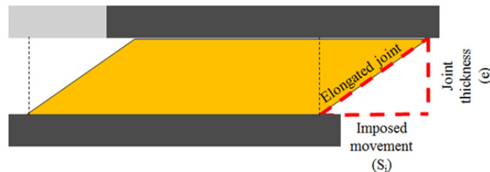
Fig. 8 Shear deformation of the joint.
