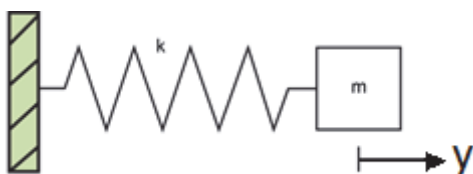
Fig. 8: simplified analogy between a mass spring system and a plate deformation under external load
