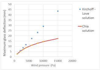
Fig 7: Comparison between the Chia solution (equation 10) of the Von Karman equation of an isotropic plate submitted to a transverse load and the approximated Kirchhoff-Love solution (equation 7)
