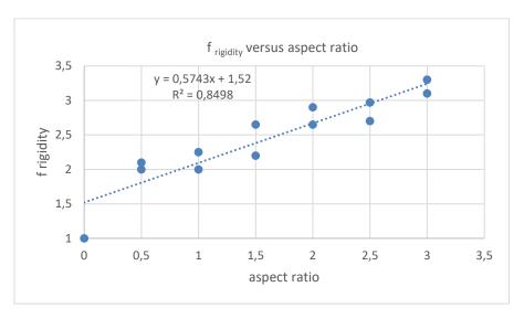
Fig. 4: rigidity factor as a function of aspect ratio using all the measured H pieces
