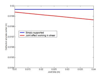
Fig.8:Calculation of the contribution of the joint working in shear on the maximum value of the glass plate deflection at its center change image
