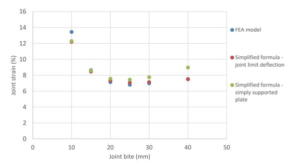
Fig. 10: comparison of maximum value of joint strain as a function of sealant bite for 3D FEA and simplified methods.
