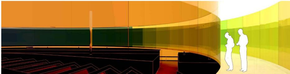
Figure 2: View of the inner appearance of the glass walls, no structural elements are in the inner and outer walls except the curved glass panes.
