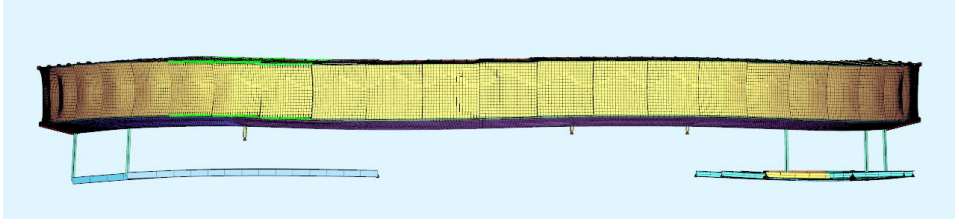
Fig. 13: Shell element model of one half of the walkway under maximum loads, displacements are scaled up.
