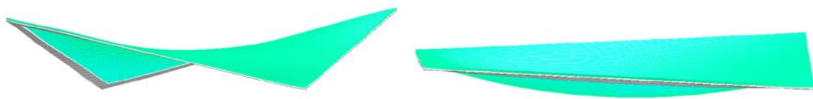
Fig. 8 Load step I: cold bending (left), load step II: cold-bent model under pressure load (right).
