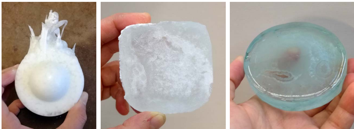
Fig. 7 a) PPG Starphire kiln-cast at 860^\circ\text{C} and mechanically quenched, b) PPG Starphire sample kiln-cast at 1.200^\circ\text{C} with top surface crystallization, c) PPG clear float sample kiln-cast at 1.200^\circ\text{C} .
