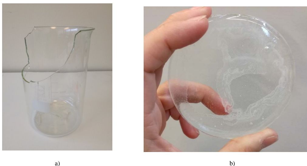
Fig. 14 a), b) Borosilicate labtube before and after casting at 1.200°C.
