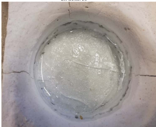
Fig. 18 Result of the lead crystal and float glass combination, fired at 1.200°C. The cracks of the mould correspond to those found in the glass.
